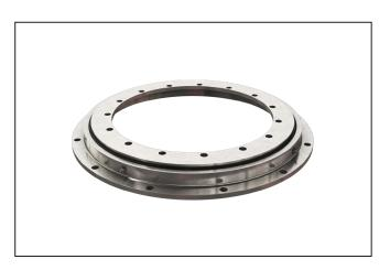
Rolling element anti-friction bearings rely on ball and raceway surface lubrication. A thin film of oil or grease should be used. Be sure not to contaminate the lubricant used in the bearings. Our standard open (unsealed) bearings are shipped with only a light oil as a corrosion inhibitor. You must lubricate these bearings with the appropriate grease or oil for your application. Sealed bearings are shipped as standard practice with 20% - 30% fill of MIL-G-81322 grease.
